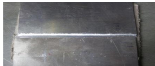
Figure-6 tensile specimen for test
